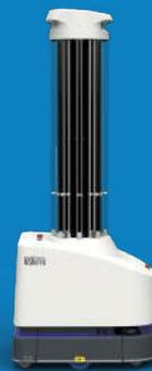
As the robot drives by it delivers approximately **70mJ/cm<sup>2</sup> of UV-C**
